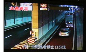
Figure 9 - Automatic Incidents Detection System
