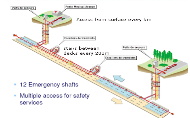
Figure 6 – overall view of the escape routes
