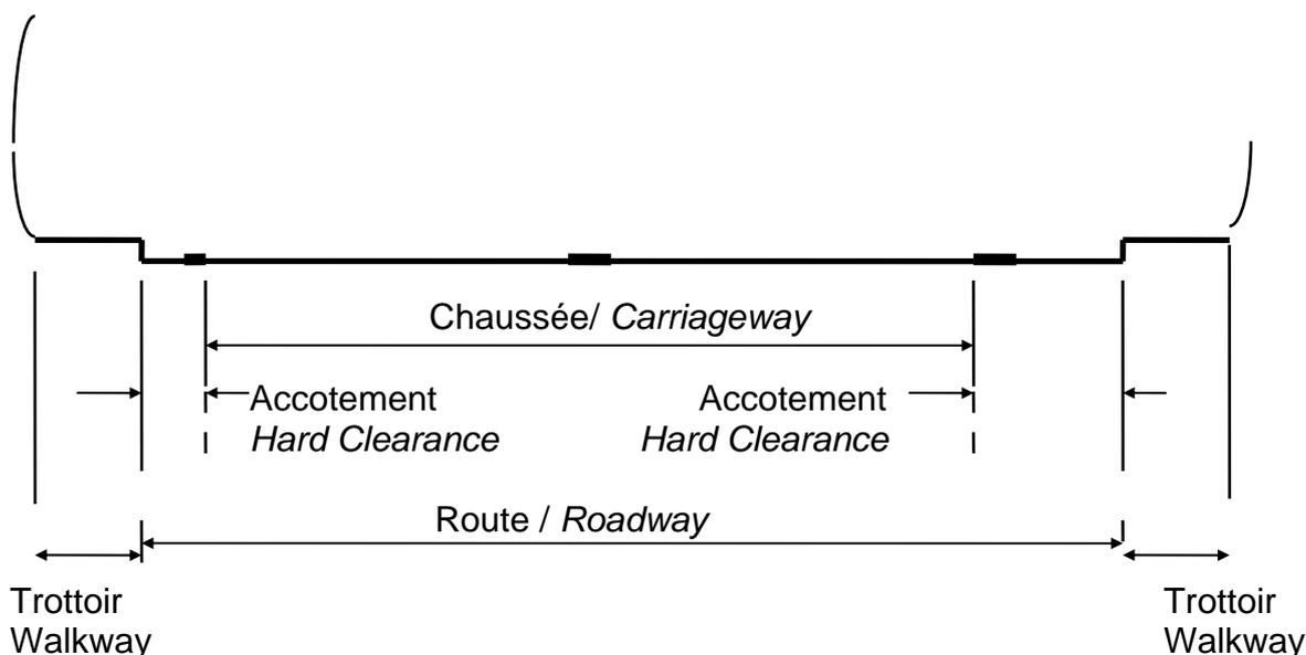
**Figure 2-2: Configuration secondaire de la plate-forme et configuration de la route / Secondary partition of the platform and partition of roadway**
