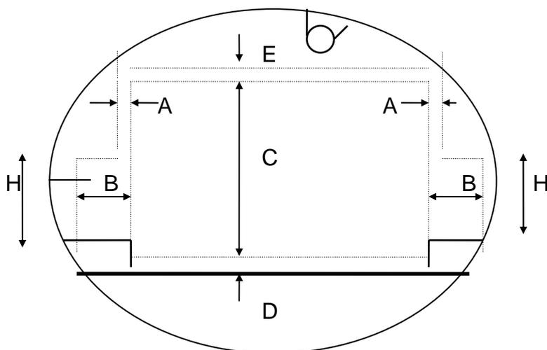
**Figure 2-5: Clearances and Allowances for Arch Profiles**
