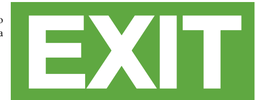
Figure 47: The proposed panel to indicate doors opening to the "safe tube" or open area
