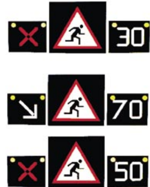
Figure 55: Clearing the overtaking lane according to the procedure adopted in the Westerschelde Tunnel (the Netherlands)
